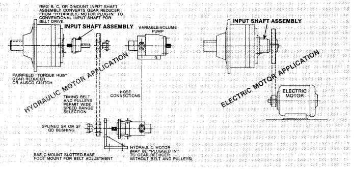
Most Fairfield and Ausco transmission equipment is installed with the axis horizontal. When this equipment is installed with the axis VERTICAL and the input shaft assembly ABOVE the gear reducer or clutch, special provisions must be made for lubrication. Contact RMG factory office for details.
